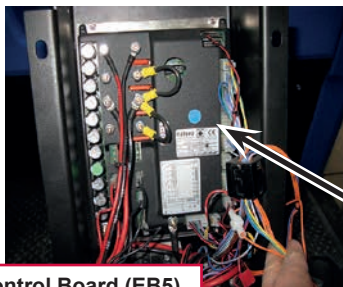
Side Main Control Board (EB5)
