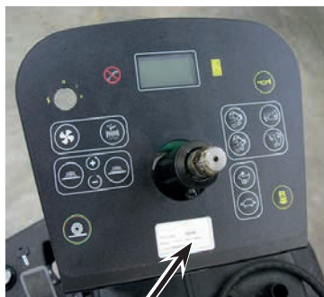
Main Control Board (EB4)
