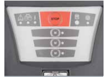
Membrane switch keypad with LED indicators
