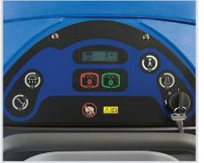
**Simple operation** Single touch button control sets proper operation of all functions, simplifying training and allowing consistent use of all operations.
