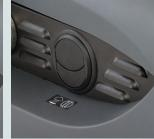
Wet sweep bypass protects the filter from water fouling when sweeping in wet conditions.
