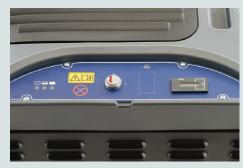
Control panel with key switch, battery charge indicator and hour meter.
