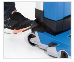
**Foot Activated Controls**Machine functions stop when in the upright position.
