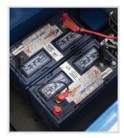
Battery Compartment The SA40<sup>™</sup> is available with wet or AGM maintenance-free batteries.
