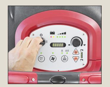
Turn on the key and verify there is enough battery power to complete the work. Charge batteries if required.
