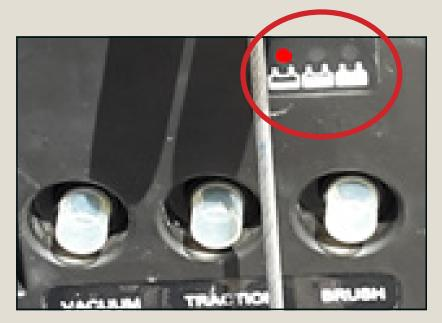
Daily: if the battery indicator shows red, put the machine on charge. Battery should be on charge if empty, not in use or if not being used for coming 8-10 hours.
