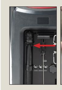
Daily: Empty the recovery tank using the recovery empty hose. Bend the soft part before removing the cap to control the flow.
