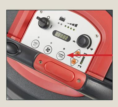
On disc version, the brush/pad holder can be removed automatically by raising the deck with the pedal and then press the click off button.
