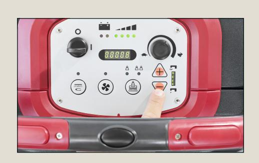
Press the + or – solution buttons to increase / decrease the water flow rate or to turn solution off.
